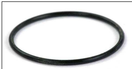
Fig. 9: O-ring after 5000 mating cycles
