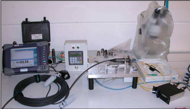
Fig. 6: measuring setup for durability and lifetime test
