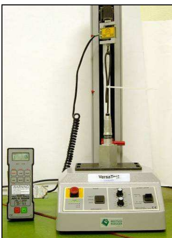
Fig. 4: Equipment for examination of cable retention
