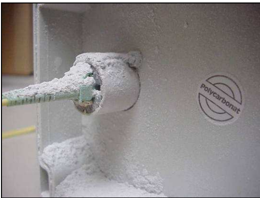
Fig.20: Dust sediment on the rear side of the receptacle after 60 min.
