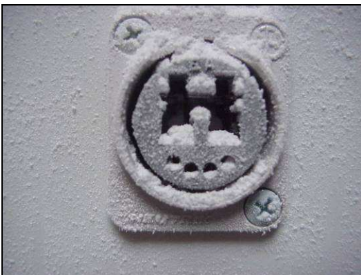
Fig. 21: Dust sediment on the front side of the receptacle after 60 min.
