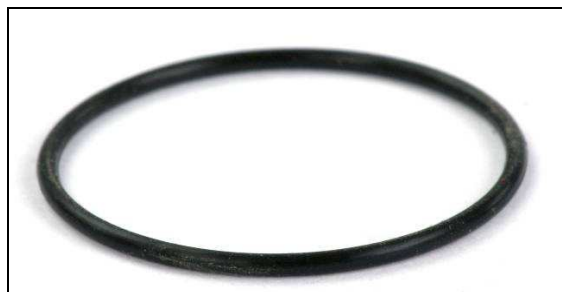
Fig. 15: O-ring after 5000 mating cycles
