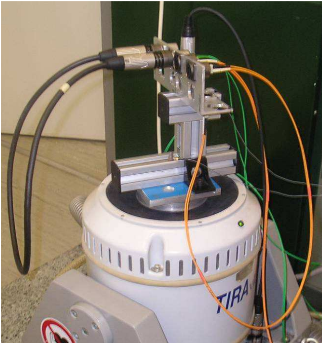
Fig. 3a: Vibration equipment and test cable arrangement
